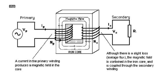
Figure 1.1 - Essential Workings of a Transformer
