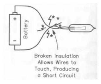
Therefore a short circuit will have too much current flowing through it. What's the best way to stop a short circuit from doing damage (because it is drawing too much power from the source)? By using a fuse. Fuses are designed to work up to a certain amount of current (e.g. 1 amp, 15 amps, ...). When that maximum current is exceeded, then the wire within the fuse burns up from the heat of the current flow. With the fuse burnt up, there is now an "open circuit" and no more current flows.
