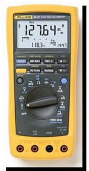
Potential difference (voltage) is measured with a voltmeter, the voltmeter is connected to a circuit under test **in parallel with the circuit**.
