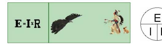
Voltage:  $E = I \times R$  (Volts) Current: I = E / R (Amps) Resistance: R = E / I (Ohms)
