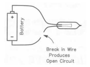
You probably figured that since there are "open circuits" that there are probably also "closed circuits". Well, a closed circuit is when the switch is closed and current is allowed to flow through the circuit.
