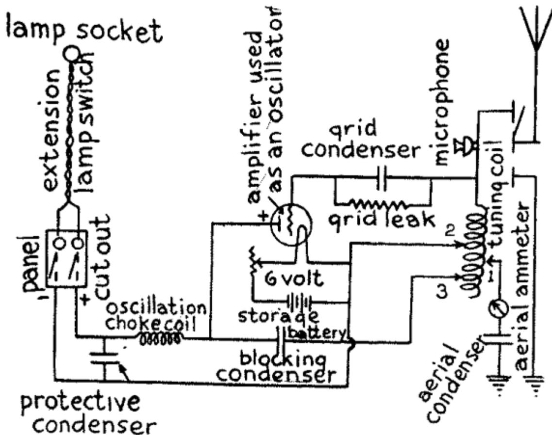
FIG. 85.—Wiring Diagram of Short Distance Wireless Telephone Set.
