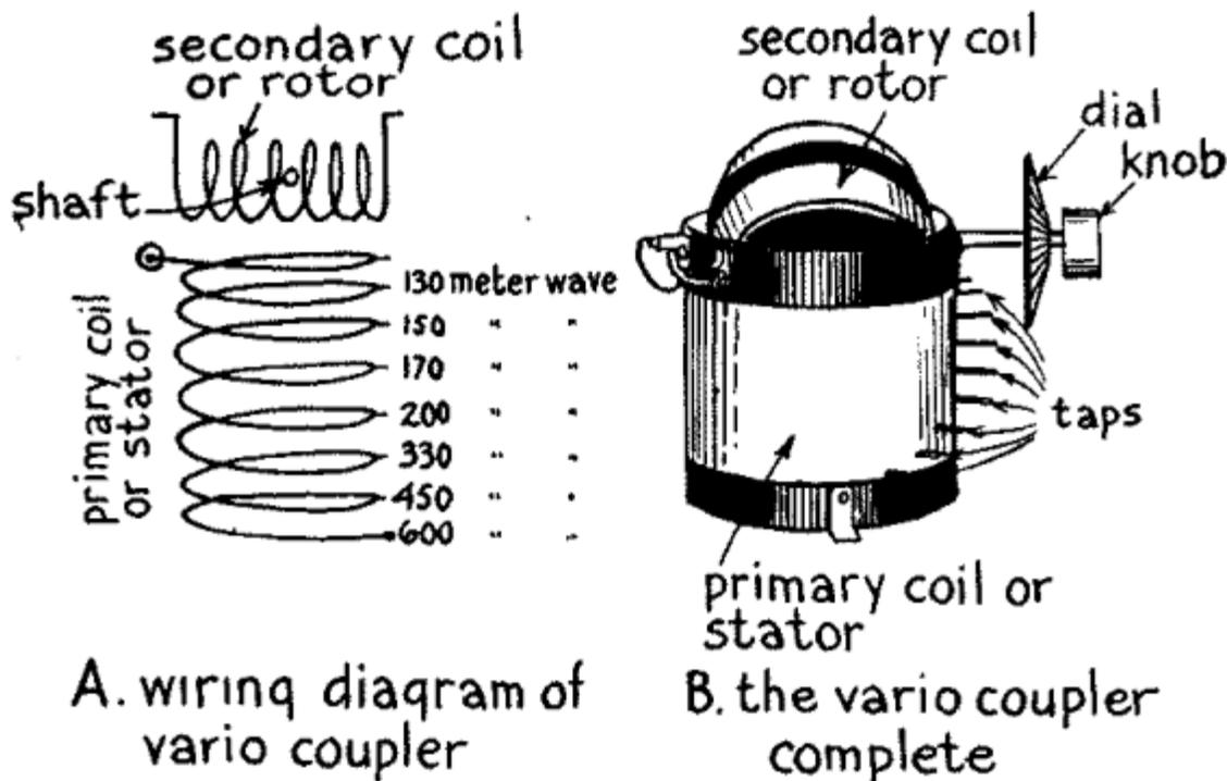
FIG. 53.—How the Variocoupler is Made and Works.
