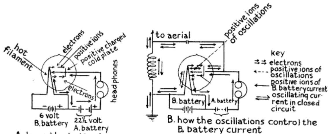
A. how the batteries are connected in
