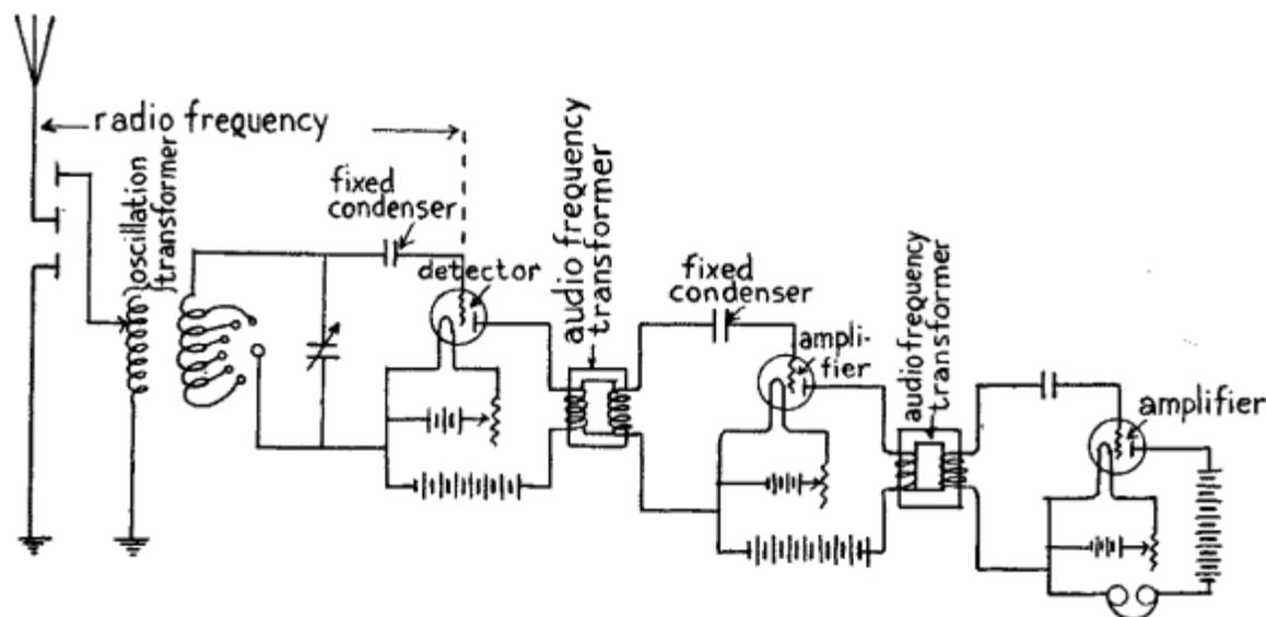
(B) FIG. 46.—Wiring Diagram for an Audio Frequency Transformer Amplifying Receiving Set.
