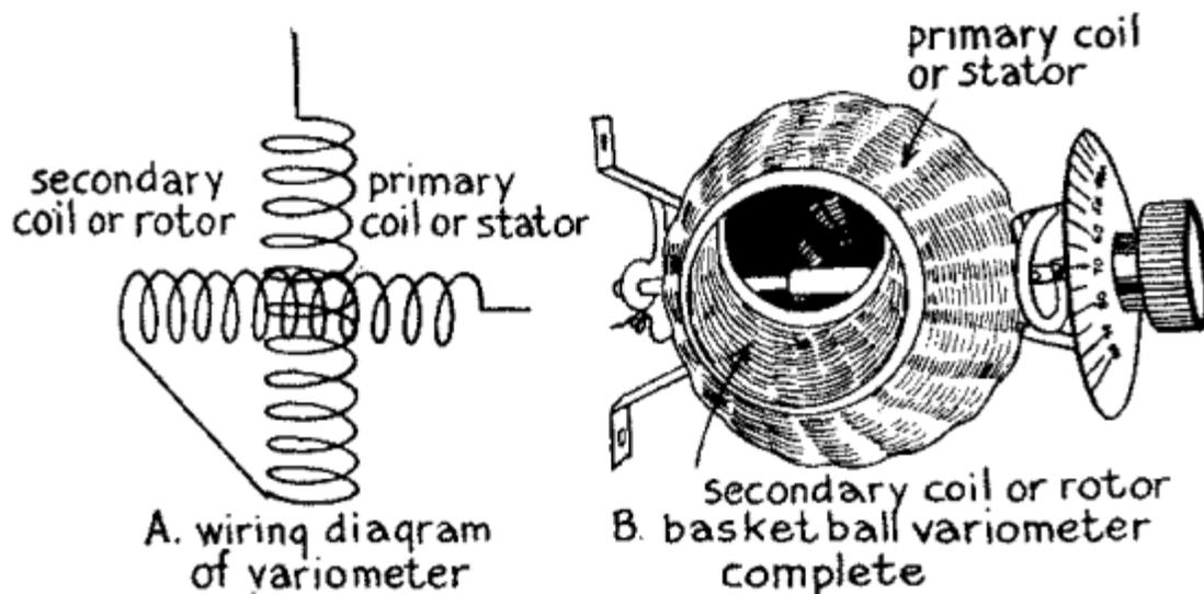
FIG. 54.—How the Variometer is Made and Works.
